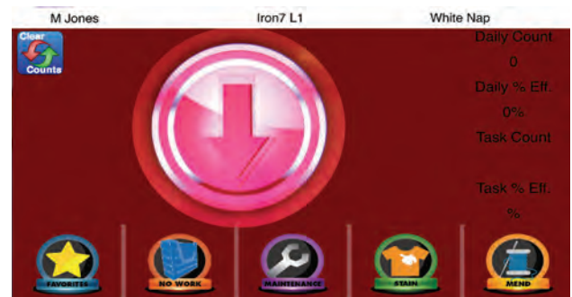
Figure 89. PPS Monitor Station. Unsatisfactory production level turns the screen red.
