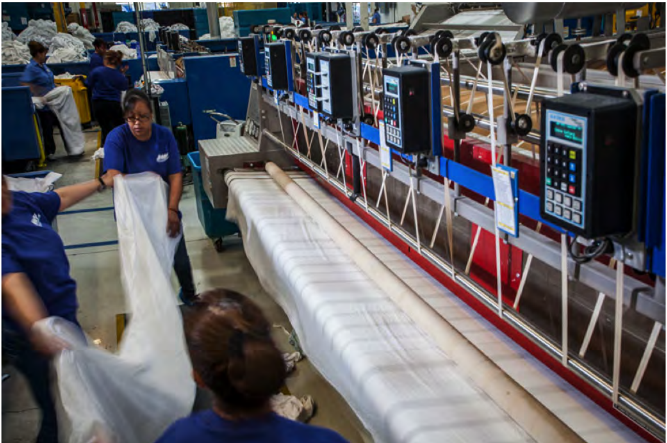
Figure 2. Workers at a roller press. The workstation is set up for either five individuals to work side-by-side logged into their own PPS monitor (photo is of a workstation using classic monitors instead of touchscreen) or logged into a group task using the Team Station. This group is logged into the Team Station performing a three-person task.
