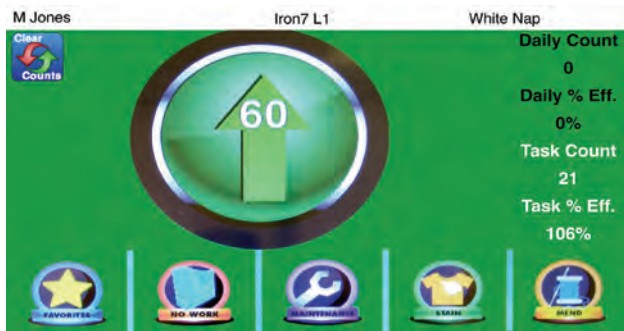
Figure 88. PPS Monitor Station. Satisfactory production level turns the screen green.
